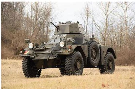
In 1949, the British Army approached Daimler to upgrade its World War Two light armoured vehicles. Having previously designed the Dingo Scout Car, Daimler created the Ferret. The Ferret was a development of the Dingo design, but it had more interior space for the crew, and could be fitted with an optional small machine-gun turret.
